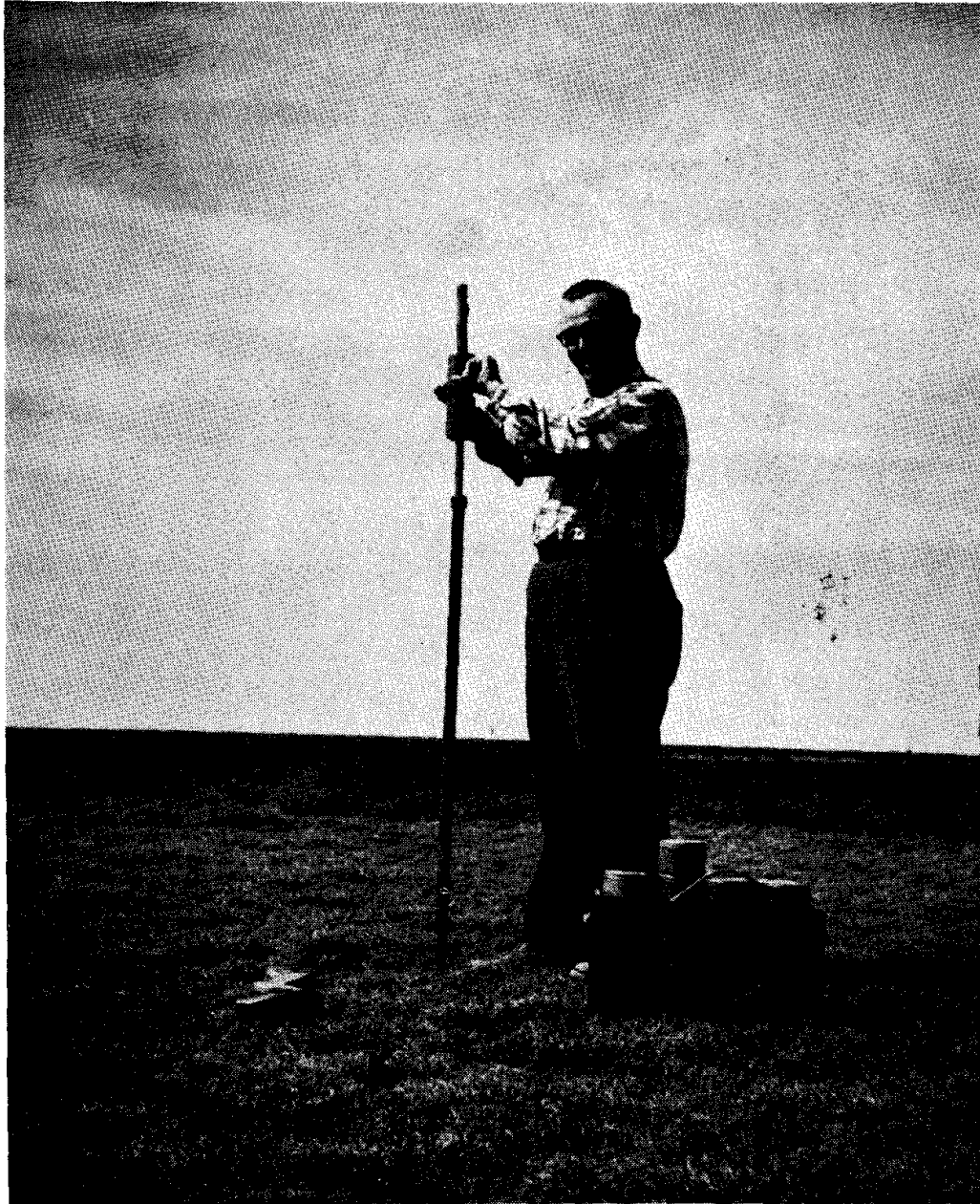
Fig. 51.--Taking soil samples for moisture determinations. "Soil moisture studies have been a part of the dryland agriculture experiments during the entire period, starting in 1914."
