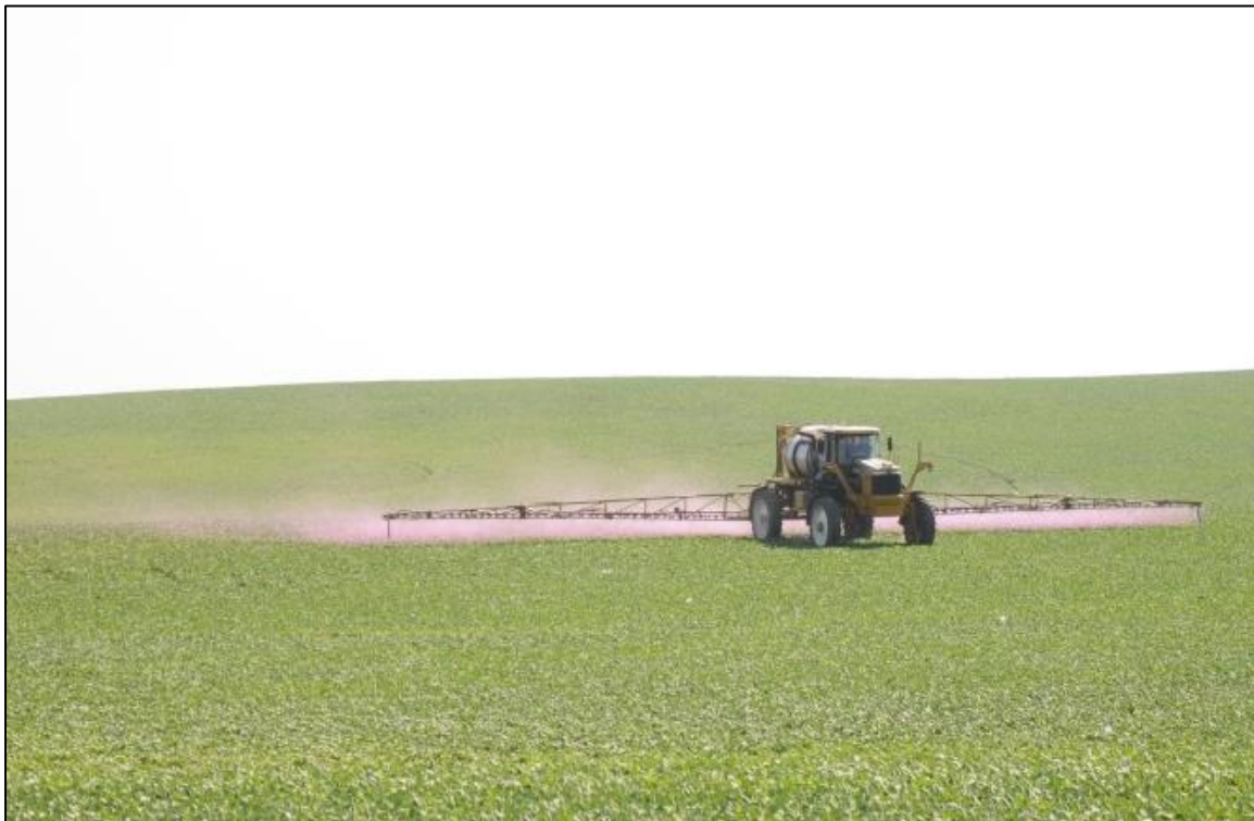
Figure 1. A spray application in 15 mph winds with nozzles producing fine droplets using a red dye to aid in visualization of the herbicide loss due to drift.
