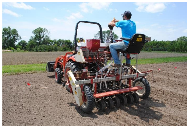
Figure 1. Hege 1000 grain drill for planting hemp variety plots.
